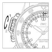
First set the depth gauge to a value below zero (for example –2 metres).
