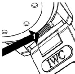
Your Aquatimer Chronograph comes with a patented IWC bracelet quick-change system that enables you to change the bracelet or strap quickly and simply, without the use of tools. To remove the bracelet or strap, use your thumbnail to firmly push the retaining lever (1) located on the underside of the horns outwards.
