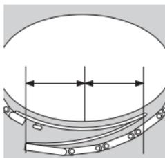
Place the watch around your wrist with the folding clasp closed, and use the overlap to estimate the number of surplus bracelet links you can now remove as described below. If you need to take out several links, we recommend removing the same number of links from each side of the bracelet
