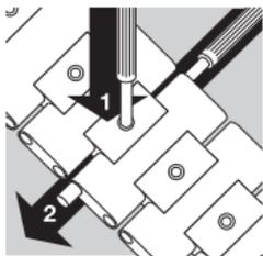
Open the folding clasp by pressing the buttons on the side. Lay the bracelet face down on a firm base. To avoid scratching the bracelet and base, place a cloth underneath the bracelet. Using the special tool provided, you can now push down the fixing bolt at the desired point of separation (1)
